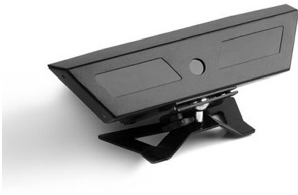
Figure 21. Example of a remote eye tracker optics module using stationary wide angle optics. Sensor, lens, and illumination components are within the enclosure. (Courtesy of Tobii Tehnology AB, Stockholm, Sweden.)
