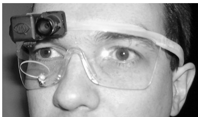
Figure 17. The head mounted module directly over the subject's right eye contains both a camera and illuminator, which are aimed down at the tilted, hot mirror beam splitter. The camera views a reflection of the eye from the hot mirror. The module just to the nasal side of the eye camera module is a scene camera, aimed toward the subject's field of view. (Courtesy of Applied Science Laboratories, Bedford, MA.)
