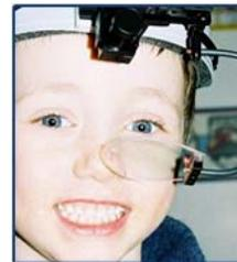
The standard (60 Hz) head mounted optics unit weighs 12 ounces (339 grams), and can be comfortably worn by participants 4 years and older. With the high-speed option (120/240/360 Hz), the unit weighs 14 ounces (395 grams).
